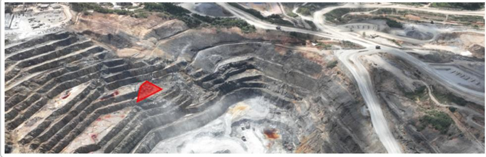
*An open-pit mine's digital twin can reveal instability in slopes before a collapse occurs. In this case, a 3D twin of the Pueblo Viejo gold mine's pit helped engineers identify a section (highlighted in red) with a low factor of safety. Continuous data updates and modeling enabled early detection of a pending slope failure, allowing for timely interventions <sup>7</sup> <sup>8</sup>.*
